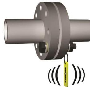
The Lamons IGT will be using UHF (Ultra High Frequency) technology, to enable users to read tags from a distance of 25 feet (860-960 MHz) using a handheld RFID reader, which is an advantage in a refinery environment. Tags will also be able to be read using QR readers from smart phones. Lamons will be writing useful information to assist with product trouble shooting, product re-ordering, and product verification installed in your flanged application.
