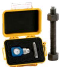
**SPC4™** load indicating fastener technology allows installation of a bolted assembly with confidence. Users can monitor the clamp load of any SPC4 bolted joint whether static or dynamic, by attaching an indicator datum disc located on the end of the fastener and reading the value with a user-friendly mechanical indicator.
