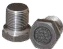
**HeaderKamm™** sealing plugs are engineered for air-cooled heat exchanger applications (ACHE) in the up and down stream markets. The plug uses an integral seal design under the bolt head, a proven Kammpro LP1 machined seal faced with inhibited graphite. This design integrates the gasket needed to seal with the plug itself reducing leak paths. The Kammpro serrations effect a seal even with imperfect surfaces solving costly installation delays.
