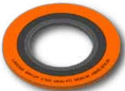
Lamons style **WRI-LP** is designed to engage the sealing surface of flanges completely from the OD to the bore. This field-proven design provides protection of the flange facings while requiring a low load for seating and maintaining an effective seal. These gaskets are recommended for use in new and undamaged flange facings. Various winding, core and facing materials are available for maximum corrosion resistance.
