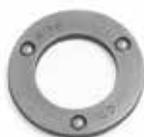
The **Ball Lock Washer** is a hardened washer which employs the use of hardened steel ball bearings that embed and grip into the flange face and nut bearing surfaces. This mechanical lock begins to occur during the hand tightening stage and is maintained throughout the tightening process. The result is a technology that eliminates the need for a back-up wrench and the need for an operator to place his hands and fingers at risk in a pinch point zone.
