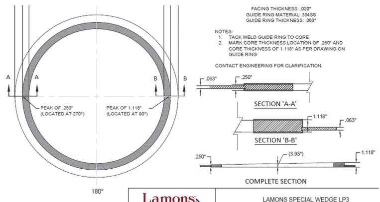
*Kammpro wedge gaskets are designed to address flanged connections where one or both flanges have fallen out of parallelism. The unique angled profile of the Kammpro core allows for even compression without the load loss required to straighten flanges.*
